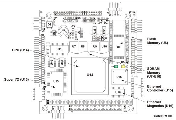
Figure 2-3. CoreModule 420 (Top View)
